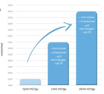
Based on: Round bale 1,20 m, 6 layers of film, 55 % overlap, 70 % pre stretch, when comparing 1500 m/25 $\mu$  film.
